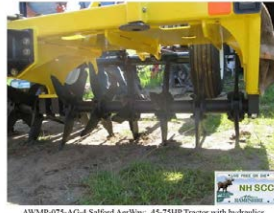
AWMP-075-AG-4 Salifed AerWay. 45-75HP Tractor with hydraulics recommended. Cultivation width 7.5'. Weight 2150 lbs.
