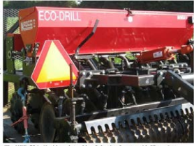
The KLEB-72 is 6' wide and capable of planting 9 rows, with 8" spacing. KASCO recommends a 25hp+ tractor, with sufficient lift capacity to handle approximately 1600 lbs. on back.
