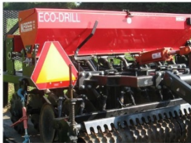
The KED-72 is 6' wide and capable of planting 9 rows, with 8" spacing. KASCO recommends a 35hp+ tractor, with sufficient lift capacity to handle approximately 1600 lbs. on back.
