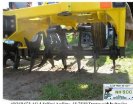
AWMP-075-AG-4 Salford AerWay - 45-75HP Tractor with hydraulics recommended. Cultivation width 7.5'. Weight 2150 lbs.
