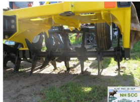
AWMP-075-AG-4 Salford AerWay - 45-75HP Tractor with hydraulics recommended, Cultivation width 7.5', Weight 2150 lbs.
