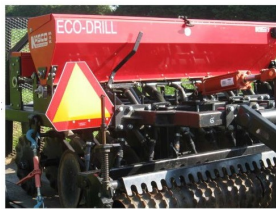
The KEDS-72 is 6' wide and capable of planting 9 rows, with 8" spacing. KASCO recommends a 35hp tractor, with sufficient lift capacity to handle approximately 1600 lbs. on back.
