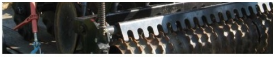
The KED-72 is 6' wide and capable of planting 9 rows, with 8" spacing. KASCO recommends a 35hp+ tractor, with sufficient lift capacity to handle approximately 1600 lbs. on back.
